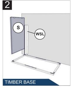
If no conrete slab / other at surface is available, use timber base frame as shown.
