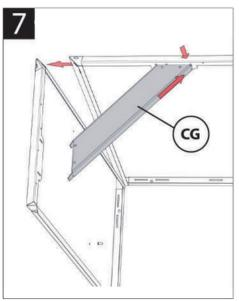
Insert corner gussets into the side and front AND side and rear panels by inserting into the corner and pushing downwards.
