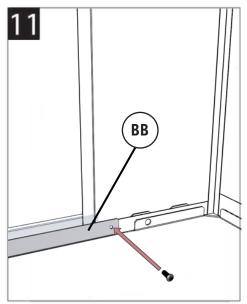
Secure Bottom Brace to Front Left and Front Right Panels with a Tek Screw.
