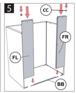
Slot Front Left and Front Right panels into the Lower Brace and Corner Brackets. Tap Corner Caps into place with a mallet.
