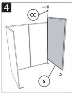
Insert the other side panel and cap. Slot Front Left and Front Right
