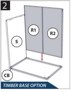
If no concrete slab / other flat surface is available, use timber base frame as shown.
