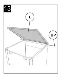
Attach top door to unit with hinge pins. Align pins with holes and tap into place with a mallet.
