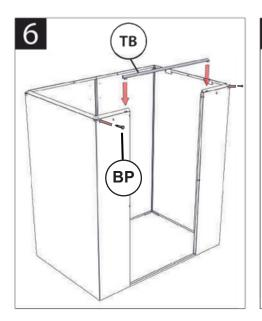
Insert Top Brace into slots in Front Left and Front Right Panels. Insert 2 x BP into slots on the front panel through the corner caps.
