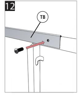
Secure Top Brace to Font Left and Front Right Panels with a Tek Screw.
