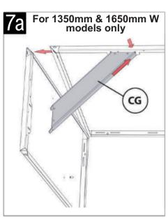
Insert Top Brace into slots in Front Insert corner gussets into the side and front panels by inserting into the corner and pushing downwards.
