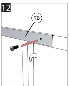
Secure Bottom Brace to Front Left Secure Top Brace to Font Left and Front Right Panels with a Tek Screw.
