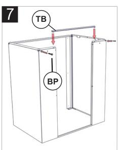
Left and Front Right Panels. Insert 2 x BP into slots on the front panel through the corner caps.
