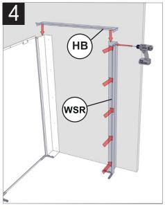
Install the Horizontal Bridge Cover, installed on the outside of the wall fixings strips. Use 2 metal tek screws to attach the horizontal bridge cover to the wall fixings strips. Fix the wall fixing strips to the wall using appropriate wall fixing anchors through the pre drilled holes.
