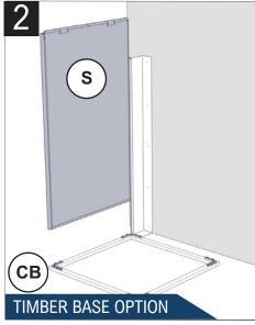
Alternatively, use timber base frame If installing on an uneven / as shown.
