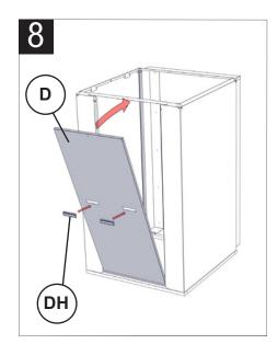
Insert the handles into the door untill a "click" is heard. Place the removable front door into the panel by placing the lip of the door over the front panel step. Insert the door by aligning the studs on the side with the slots in the front panel. Push in slightly and then down.
