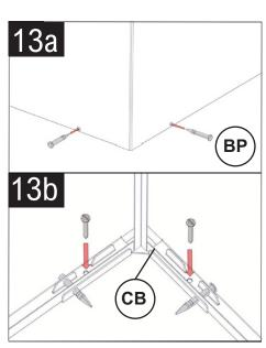
Push base pins into holes in the bottom edge of outer panels and through corner bracket (a). Anchor box to timber base frame as shown or concrete slab / other at surface (b). Do this for for all 4 corners.
