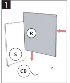
Locate slots on bottom of side and rear panels and push down into the corner brackets as shown.
