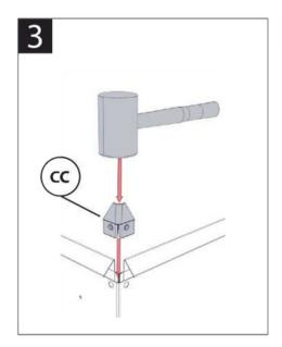
Now insert a corner cap into the holes in the top of the panel to join them. Tap into place with a mallet.
