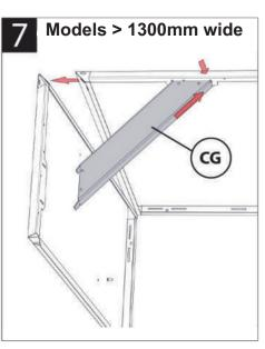
Insert corner gussets into the side and front AND side and rear by inserting into the corner and pushing downwards.
