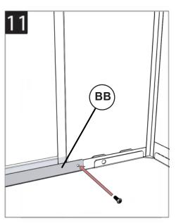
Secure Bottom Brace to Front Left and Front Right Panels with a Tek Screw.
