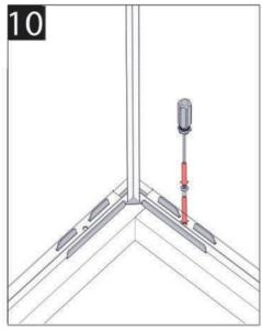
Anchor box to timber frame as shown or concrete slab / other flat surface.
