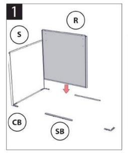
Locate slots on bottom of side and rear panels and push down into the corner and straight brackets as shown.
