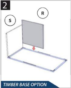
If no concrete slab / other flat surface is available, use the timber base frame as shown.
