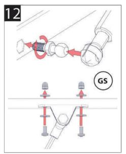
Attach gas struts to the side panel by attaching ball bearing first. Now push the struts onto the ball bearing. Insert bolt and washer into the faceplate of the strut and through the predrilled holes in the top door and secure with the dome nuts provided,
