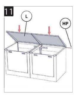
Attach the lids to unit with hinge pins. Align pins with holes and tap into place with a mallet.
