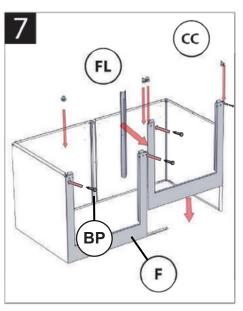
Slide the front panels into position and insert the filler and caps (same method as for rear panels). Insert 4 x BP into slots on the front panels through the corner caps.
