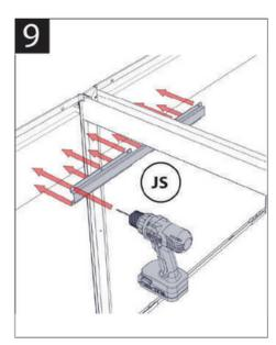
Get the joining stiffener and screw fix to timber panels.
