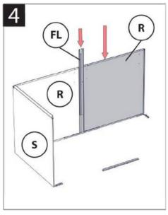
Now insert the other rear panel onto the tabs of the corner and straight brackets. Insert the filler between the panels and slide into the straight bracket, ensuring slots at top of filler are in line with slots at top of panels.
