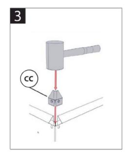
Now insert a plastic cap into the holes in the top of the panel to join them. Tap into place with a mallet.
