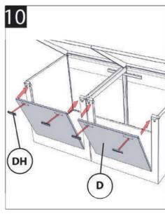
Insert the handles into the door untill a "click" is heard. Place the removable front door into the panel by placing the lip of the door over the front panel step. Insert the door by aligning the studs on the side with the slots in the front panel. Push in slightly and then down.
