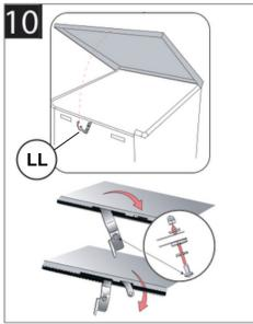
Insert staple into slot into top lid by pinching sides.
