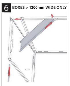
Insert corner gussets into the side and front panels by inserting into the corner and pushing downwards. Remove metal dowel if applicable to your model.
