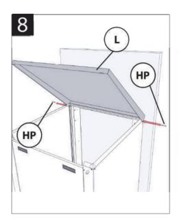
Attach lid to unit with hinge pins.
