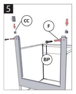
Slide front panel onto corner brackets. Insert the last 2 caps and insert 2 x BP into slots on the front panel through the corner caps. If you have >1.3m wide models, see step 6 before inserting caps.
