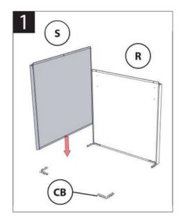
Place slots on bottom of side and rear panel and locate on slots on corner brackets.
