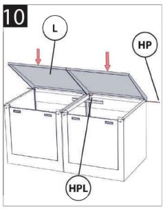
Get the joining stiffener and screw Attach the lids to unit with hinge pins. Align pins with holes and tap into place with a mallet. For the central join, tap the centre hinge pin through both top lids and corner caps.
