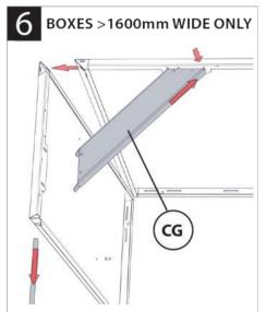
Insert corner gussets into the side and front panels by inserting into the corner and pushing downwards. Remove metal dowel if applicable to your model.
