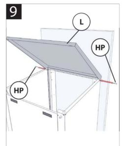
Attach lid to unit with hinge pins. Align pins with holes and tap into place with a mallet. Insert door latches into slots in lid.
