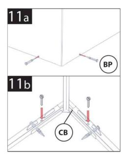
Push base pins into holes in the bottom edge of outer panels and through corner bracket (a). Anchor box to timber base frame as shown or concrete slab / other flat surface (b). Do this for for all 4 corners.
