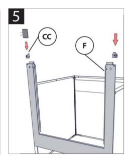
Slide front panel onto corner brackets. Insert the last 2 caps. If you have >1.6m wide models, see step 6 before inserting caps.
