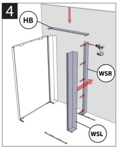
Now insert the other wall fixing strips onto the tabs of the corner and straight brackets. Screw horizontal bridge cover into Left and Right Wall Strips.
