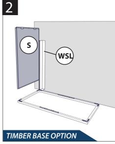
If no conrete slab / other flat surface is available, use timber base frame as shown.
