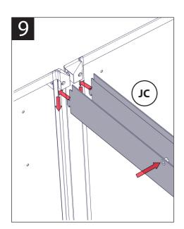
Now it's time to attach the joint channel into the rear and front panels. Push tabs into the slots (through fillers and rear/front panels) and then push down to lock. Ensure joint channel nut is orientated towards the rear as shown.
