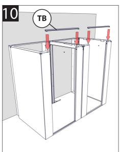
Insert Top Brace into slots in Front Left and Front Right Panels.
