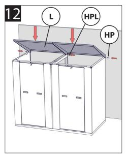
Attach lids to the unit with hinge pins. Align pins with holes and tap into place with a mallet. For the central join, tap the centre hinge pin through both top lids and corner caps.
