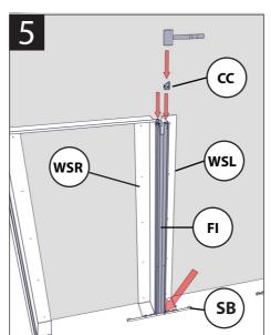
Insert the filler between the panels and slide into the straight bracket, ensuring slots at top of filler are in line with slots at top of wall fixing strips. Place the plastic caps into the wall fixing strips to join them to the filler.
