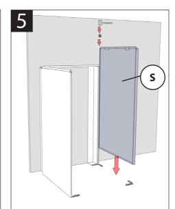
Align the slots int the front panel and slide into postion. Insert the last 2 caps.
