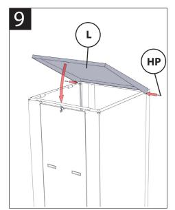
Attach top door to unit with hinge Attach the latch to the door using pins. Align pins with holes and tap into place with a mallet.
