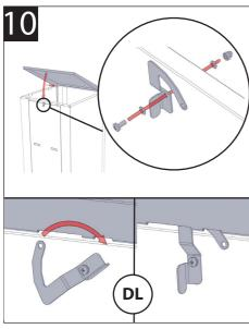
the supplied screw/washer/nut as per above. Rotate the Latch clockwise to "lock" into the top lid.
