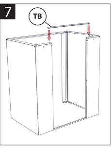
Insert Top Brace into slots in Front Left and Front Right Panels.
